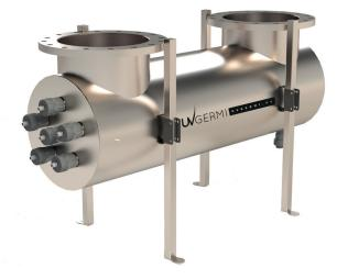
The **UVDECHLO FD600** reduces the level of combined chlorine in swimming pools through a photochemical action on all organochlorine compounds found in the water (monochloramine, dichloramine trichloramine). It also destroys Giardia and Cryptosporidum.
